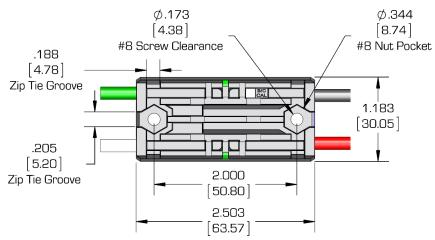
The Victor SP can be mounted using either (2X) #8-32 screws or zip-ties. The Victor SP's aluminum case is electrically isolated from the electronics, meaning it is safe to mount directly to a robot's frame!
