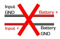
To power the Victor SP, connect the positive input (red) wire to the selected positive terminal of the Power Distribution Panel (PDP), and the input ground (black) wire to the corresponding ground terminal. In many cases, the Victor SP may be wired directly to the robot's PDP without extension cables – this is preferable since it reduces the number of electrical connections. If the robot's design does not allow for a direct connection to the PDP, extension cables may be used.
